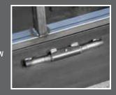
All Wagon HD models feature a reinforced wheel box structure. A 1" x 3" tube runs horizontally across the top of the wheel box and ties into two 1" x 3" vertical tubes at each end of the wheel box. Vertical tubes extend the full sidewall height - bottom rail
